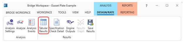
The **Analysis Results** shown below will open. This window shows the critical rating factor considering all truss members and the panel point gusset plates that were included in the analysis. The limit states specific to gusset plate are Gusset Plate Fastener, Gusset Plate Bolt Slip, Gusset Plate Tension, Gusset Plate Compression, Gusset Plate Vertical Shear and Gusset Plate Horizontal Shear. The Rating Results Summary is the only report type available.
