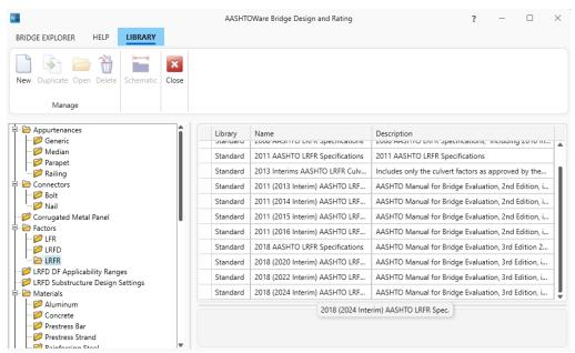
Double click on the **2018 (2024 interim) AASHTO LRFR Spec**. to open the following window and select the **Steel** tab. The gusset plate LRFR resistance factors are listed at the bottom of the table.
