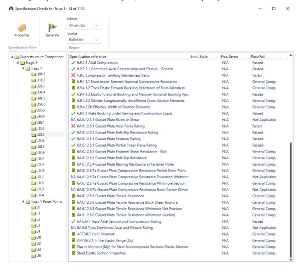
The following list of LRFR specification articles will be checked for gusset plates. The implementation of these articles is described in detail in the **AASHTO LRFR Truss Method of Solution Manual's** Appendix B.
