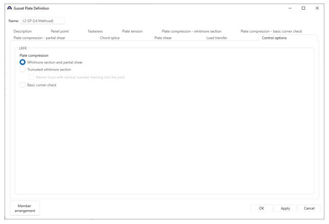
The default selection for plate compressive resistance is Whitmore section and partial shear.
