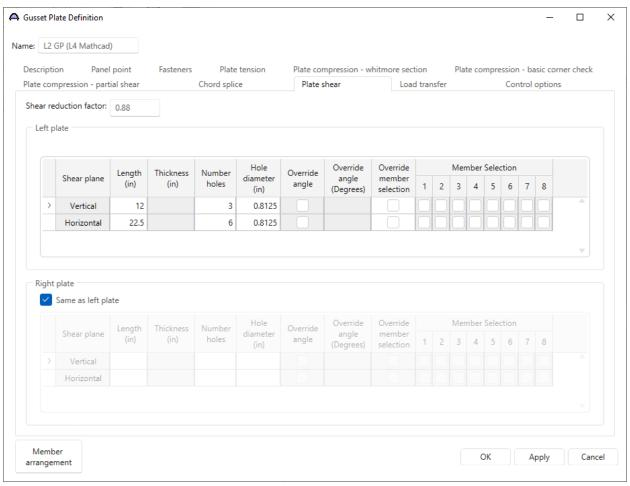
Shear reduction factor = Shear reduction factor for the gusset plate. Defaults to 0.88.
