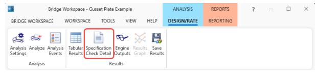
Gusset plate specification articles specific to a member and the member loads (like fasteners, tension and compression) are listed under the truss member. Gusset plate specification articles that are for the gusset plate and all loads coming into the gusset plate (like shear and chord splice) will be listed under the panel point.
