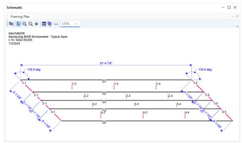
From the schematic it can be seen that the diaphragms are not entered correctly. The mid bays are incorrectly placed by the wizard. In this example, since the girders have uneven spacing, the mid-bays need to manually be fixed. The distance from the end of the left girder of the interior bays is 24'-6" + 4'-10.5" - 5'9" = 23'-7.5". Navigate to the **Diaphragms** tab of the **Framing Plan Detail** window and re-enter the data as described below.
