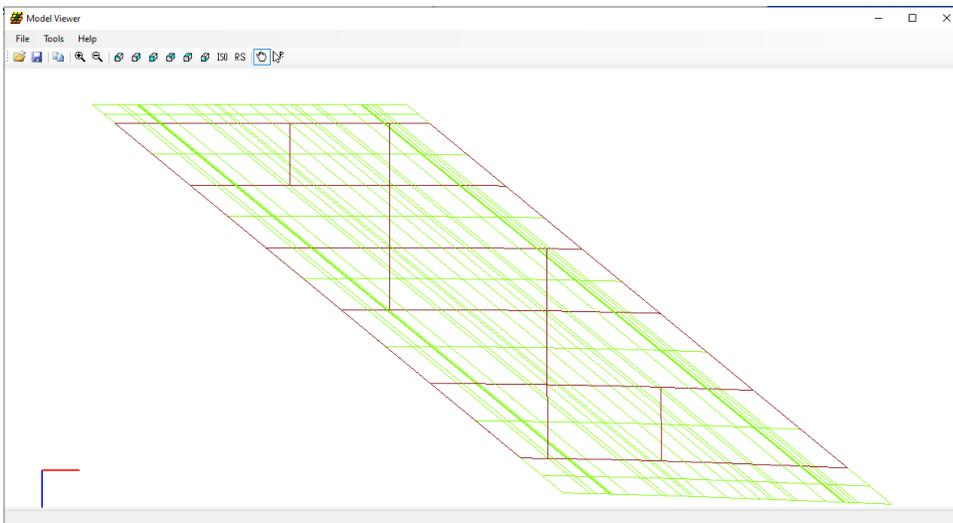
The model is improved with double the number of elements between girders. Comparing the moment for the applied uniform dead load from utilities at the first support, the computed moment is about 11.5% larger than in the first case. With such a large difference in moment, consider further mesh refinement.
