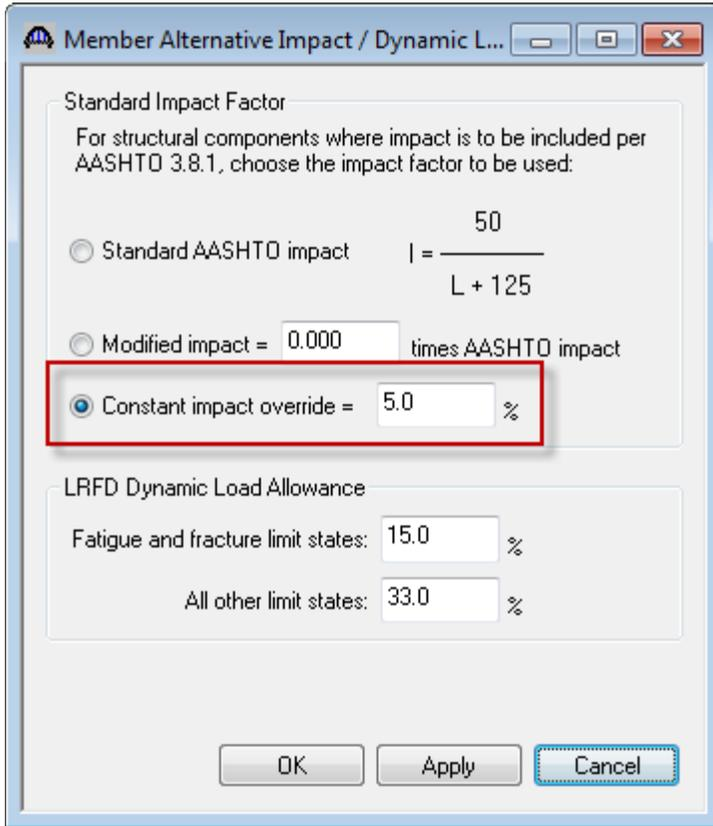
**Fig 16. Member Alternative Impact/ Dynamic Load Allowance Window**
