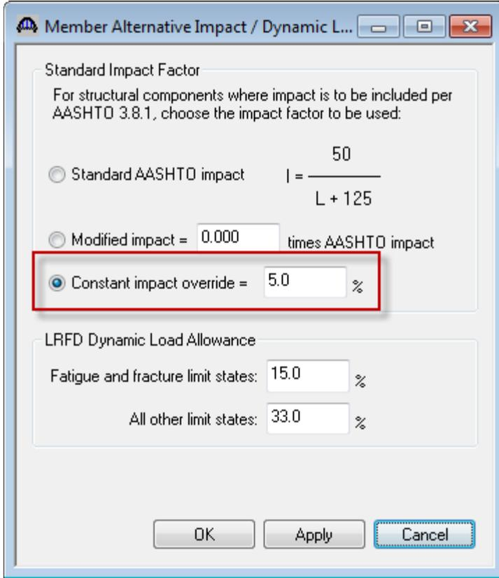
**Fig 23. Member Alternative Impact/ Dynamic Load Allowance Window**
