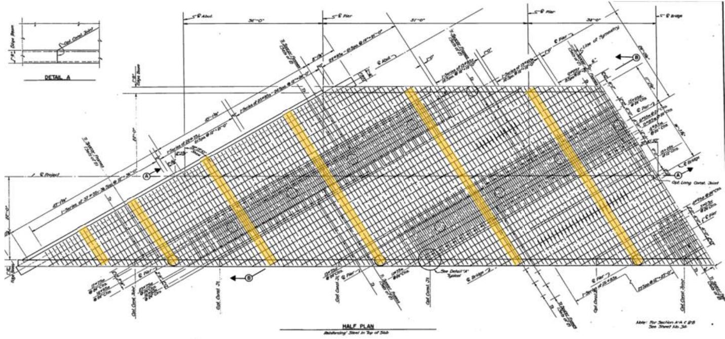
Top Slab Reinforcement
